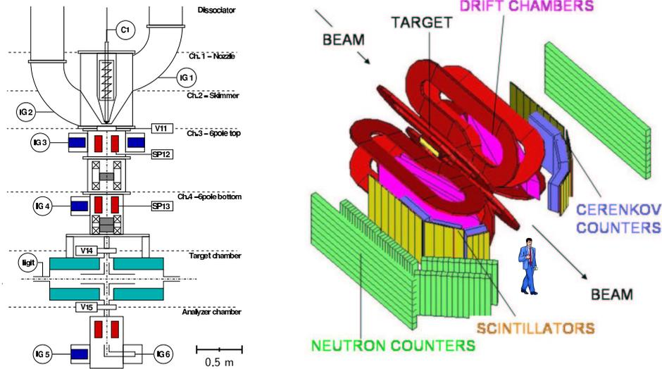
Figure 1. Schematics of the Atomic Beam Source (left) and the BLAST detector (right).
