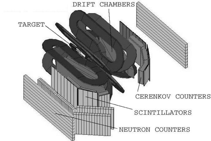
Figure 1. Schematic of the BLAST detector. In the middle are the storage cell and the eight magnetic field coils. In the order away from the target are the wire drift chambers, Cerenkov counters, time-of-flight scintillators and neutron detectors.
