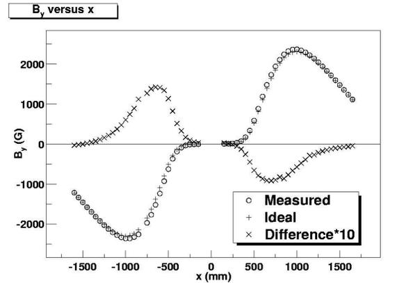
Figure 3-13: BLAST Field Map vs Biot-Savart Calculations for  $B_y$ , 500 mm downstream of the target in the midplane
