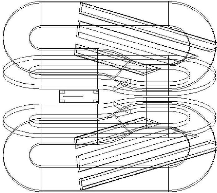
Figure 3-21: The drift chambers for BLAST are shown here in an overhead view with non-visible lines shown for display purposes
