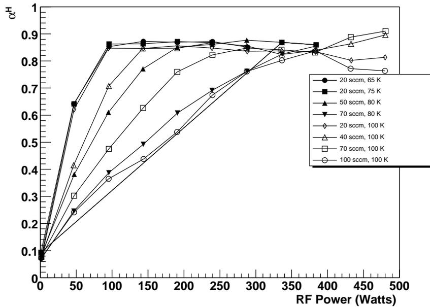
Figure 3-7: Hydrogen Atomic Fraction versus Flow Rate and Nozzle Temperature
