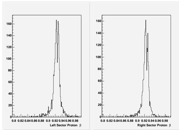
Figure 4-16: Proton  $\beta$  before cuts for BAT events
