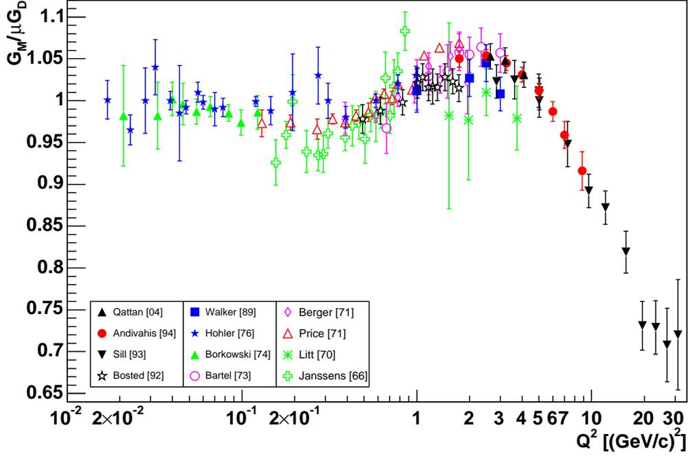
Figure 1-2: Magnetic form factor - world unpolarized data
