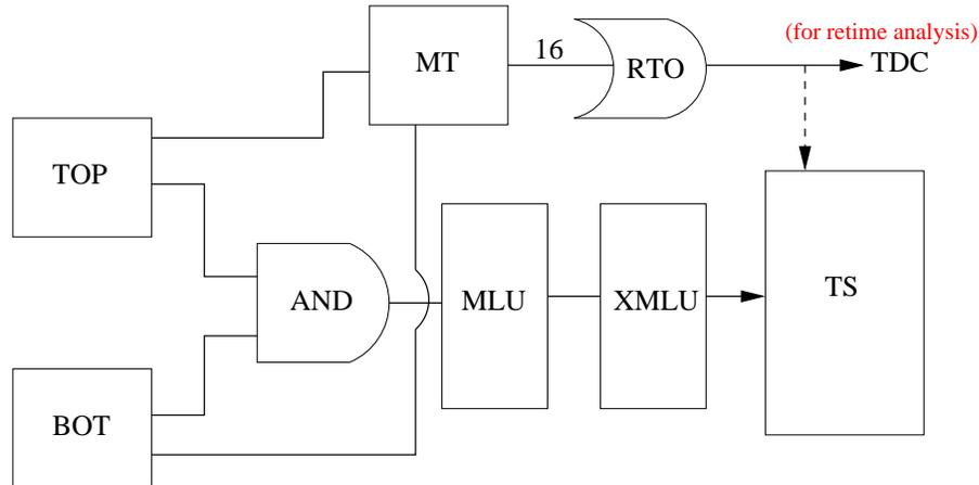
MEAN TIMER (MT): MAKES TRIGGER INDEPENDENT OF AZIMUTH
